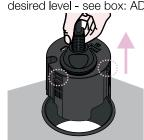
Note! Pay attention to the locking geometry as it will help with adjusting the inner part to the desired level.
